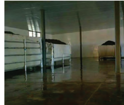
Some tea processors have recently begun piling leaves on large stainless steel bins that rest on legs several centimeters above the floor. The plates are perforated with active colonies sandwiched between layers.
