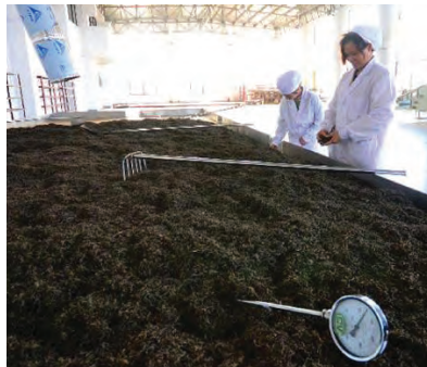
De-blocking tool(left) and a thermometer for temperature to monitor temperature(right).
