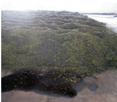
Wetted teas being piled up
